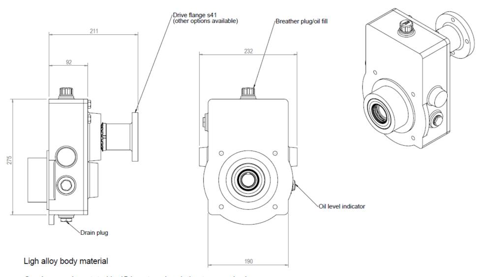
Gearbox can be rotated in 45deg steps in relation to pump body
